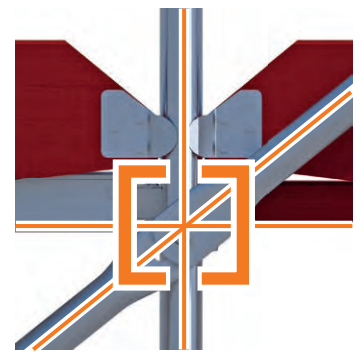
Power centre: the SUPER scaffold node makes this façade system an outstanding workplace from a statics point of view.
